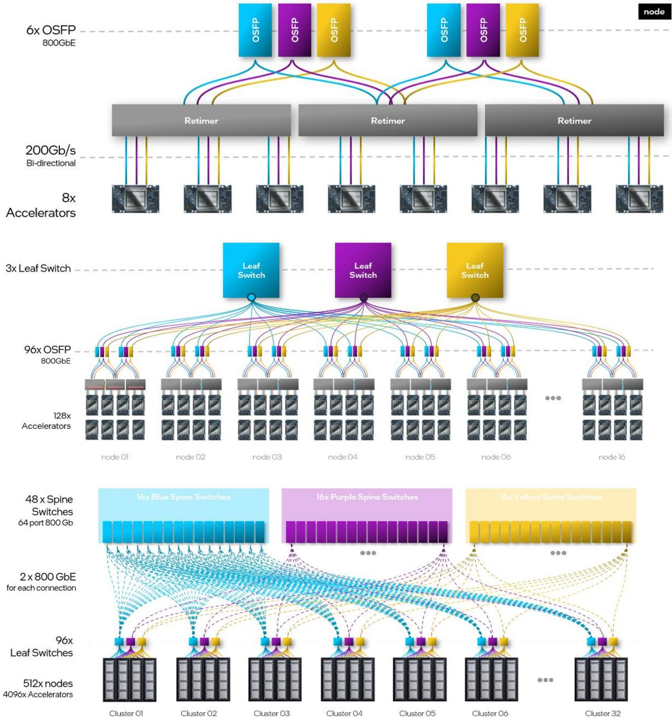
Figure 17. Intel® Gaudi® 3 Accelerator – Scale-out Cluster Architectures
