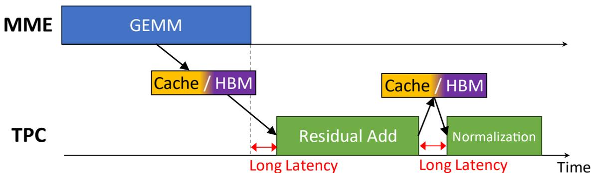
Figure 19. Illustration of timeline execution for naïve software implementation of the sub-graph in Figure 18
